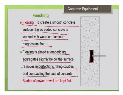
So, following screeding, the next stage is floating. So, always give some time interval between every stage of finishing and then do it. The main objective of floating is to create a smooth concrete surface. So, what you do is you either go for a wooden float like this or it may be even a metal one aluminum, magnesium, the metal floats are also available. So, with this metal float keep this blade flat and then smoothen the concrete surface.
