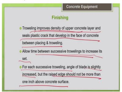
So, by troweling you can improve the quality of the upper layer of the concrete. You can improve the density of the upper layer of the concrete. If there is any crack plastic crack which is formed between the placing and the troweling. Those cracks can be filled any voids can be filled. So, troweling improves the density of the upper concrete layer and seals the plastic crack that develop in the face of the concrete between placing and troweling.
