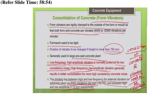
The next type of vibrator we are going to discuss is about the form vibrators. So, these are external type of vibrators. So, basically you are going to clamp your vibrator to the formwork. So, the formwork will vibrate and the vibrations will be transferred from the formwork to the concrete inside. So, this is also an indirect method of vibration. So, obviously, there will be some loss in transfer.
