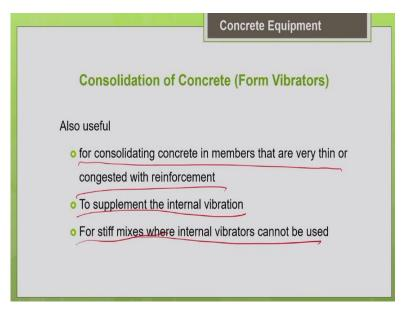
So, where do we use this form vibrators? Basically for thin sections as I told you where the internal vibration is not possible for a consolidating concrete in members that are very thin or congested with reinforcement where internal vibration is not possible. We go for form vibrators. And also in some cases to supplement the internal vibration in addition we can do the external vibration also.
