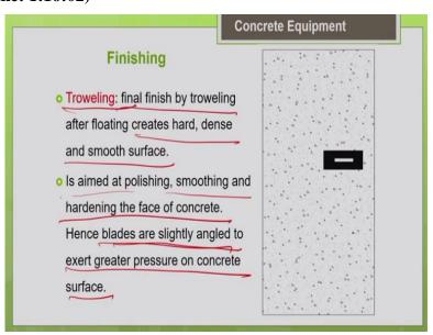
And the next step of the finishing is troweling. So, troweling, what you do? As I told you the finishing we are doing it in stages. So, troweling is also a floating only. But it refers to a different stage of floating. So, the final finish we call it as troweling. So, basically, the troweling is done after floating. So, manually when we do we are using the same tool only. But, since we are doing it in a delayed manner, so, by that time the concrete would have hardened.
