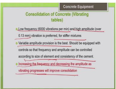
So, here also the same guideline you can apply. For stiffer mixes, go for higher amplitude. So, you go for high amplitude above 0.13 mm and you can go for low frequency less than 6,000 vibrations per minute. So, another thing is always it is preferable to have a vibrator where you have a control to manipulate the amplitude and the frequency so that you can match it corresponding to the consistency of the concrete.
