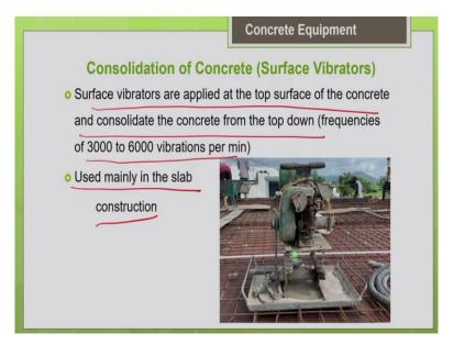
Now, let us move on to the surface vibrators. So, let us see how to do the consolidation of the concrete using surface vibrators. So, these vibrators as the name indicates the vibration is applied at the surface of the concrete and from the surface the vibration will be transferred throughout the entire depth of the concrete. So, generally speaking the internal vibrators are the best one.
