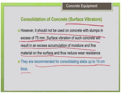
So, one thing to be noted here is this surface vibrators should not be used for a concrete with a very high workability above 75 mm. If the workability is above 75 mm for such high workable concrete mixes, we are not supposed to use surface vibration. So, what will be the major issue is when we do surface vibration for such highly workable concrete mixes, there are more chances for segregation, so, like water and thin layer of paste will come to the top surface of the concrete.
